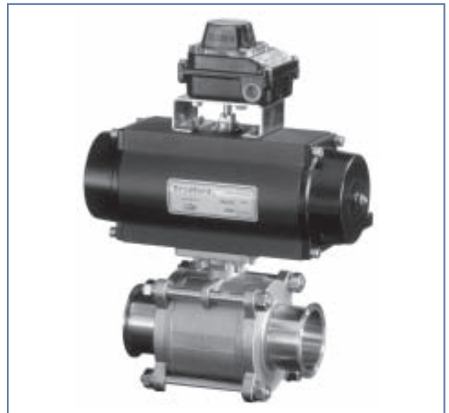
Bradford™ automated 2 1/2" 2-way encapsulated ball valve with spring return fail close actuator and NEMA 4/4X limit switch with two SPDT mechanical switches pictured. BV2CV-250CC-BFC .
