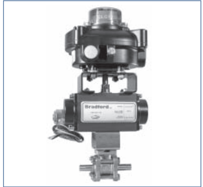
Bradford™ automated 1/2" encapsulated 2-way ball valve butt-weld ends spring return actuator and NEMA 7 (explosion proof) SPDT limit switch with two proximity switches and NEMA 7 NAMUR mount 24VDC voltage solenoid valve pictured. BV2CV-050BB-FPC .
